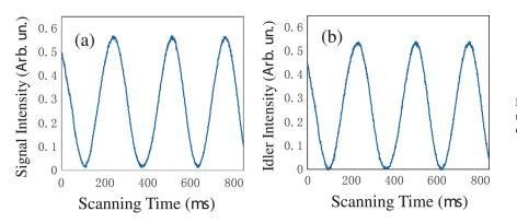
FIG. 3. (Color online) Interference fringes for the nonlinear interferometer. (a) Signal output. (b) Idler output.
