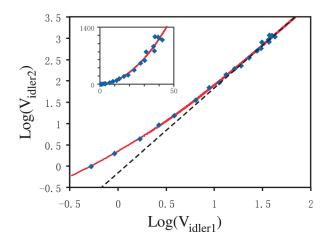
FIG. 5. (Color online) Logarithmic of the maximum intensity of the interference fringe as a function of logarithmic of the intensity of the phase sensing field inside the nonlinear interferometer. Inset: linear scale plot; red solid line: fit to the function in Eq. (11); dashed line: slope 2 for quadratic dependence.
