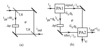
FIG. 1. (a) A linear Mach-Zehnder interferometer. (b) A nonlinear interferometer with parametric amplifiers (PA1 and PA2) as the equivalent beam splitters.
