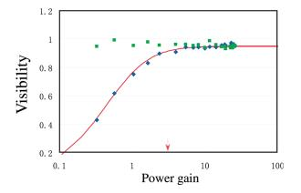
FIG. 4. (Color online) Visibility of interference fringe as a function of power gain  $|g_0|^2$ . Green squares: idler fringe; blue diamond: signal fringe; red solid line: plot of the function in Eq. (10); the function is multiplied by a factor of 0.95 for imperfect alignment. The arrow corresponds to the gain for Fig. 3.
