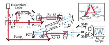
FIG. 2. (Color online) Layout for an experimental realization of the nonlinear interferometer. H: half wave plate; PBS: polarization beam splitter; AOM: acoustic optic modulator; GL: Glen laser polarizer; GT: Glen-Thompson polarizer; SMF: single-mode fiber; D: detector.
